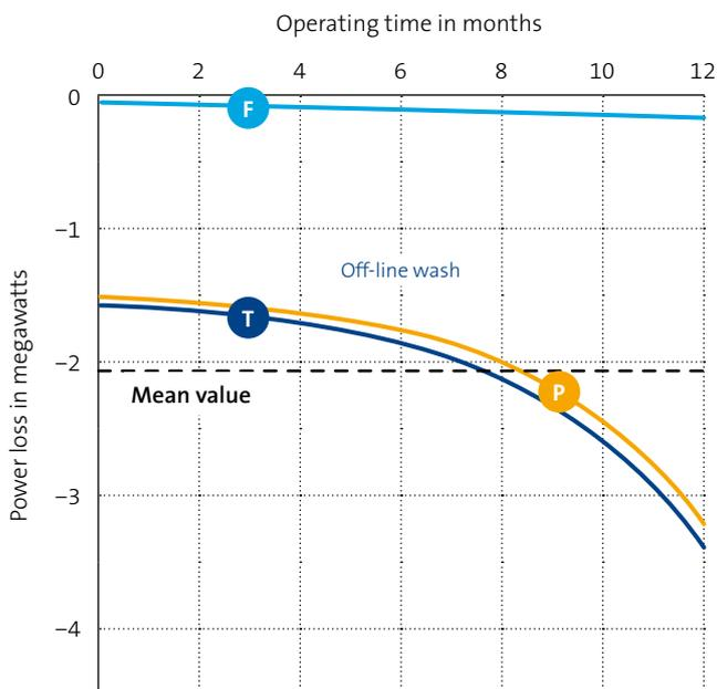
**4: Power loss with e.FFECT-optimized filter system**
