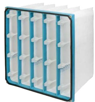
Coalescing filters offer optimal protection against penetrating water and salt, especially in offshore or coastal environments and in many other locations with high humidity. As prefilters with special drainage properties, they prevent water droplets from passing through the subsequent filter stages.
