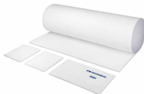
Viledon® filter mats are progressively structured, with the density of the fiber layers increasing towards the clean air side. This ensures an optimum in terms of defined filter performance and dust holding capacity, coupled with a low pressure drop. All filter mats are produced using an eco-friendly formula. We offer a range of variants for use in general ventilation and air-conditioning technology as well as for the painting industry.
