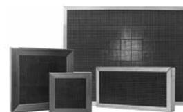
The Viledon® HM® modules are an assembly of Versacomb™ media housed in either a plastic or metal frame for removing gas-phase contaminants from outdoor or recirculated air. The module is available in nominal depths of one, two, four and six inches as standard. Viledon® HM® modules are designed to fit in a side-access filter rack or a Type 8 filter frame, and are available with or without a header.
