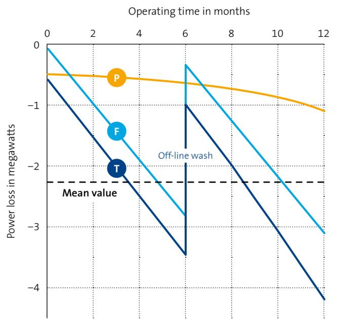
**3: Power loss with multi-stage ultra-fine filter system at high EPA level**
