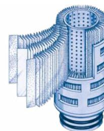
In the production of filter cartridges, Viledon® novatexx spunbonded nonwovens serve as “spacers” between the pleats on the face side and as a drainage layer on the clean side. The performance profiles of the media concerned can be very specifically designed to requirements. The nonwovens involved can be easily pleated together with the membrane without damaging the latter.
