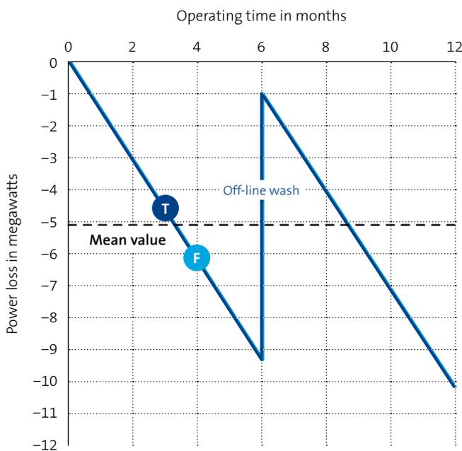
**2: Power loss with conventional, 2-stage filter system**
